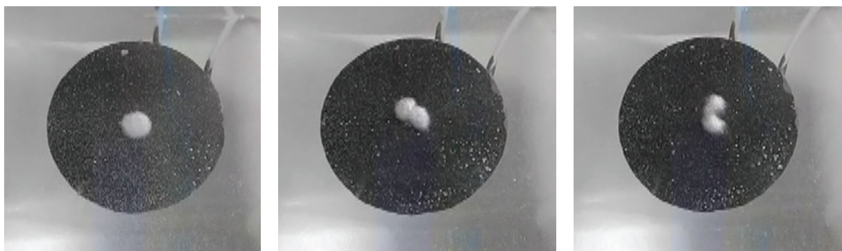
FIGURE 9. Separation of a large multibubble into two smaller sizes (left to right video footage)
